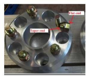
$\Delta$ Please take the time to make the install/Torque bolt in a 3 steps.
