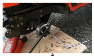
Use the supplied 🖄 tapered nut, make sure only tapered nuts are to be used to install the spacers to the axle. The factory Stud treads are 12mmx1.25 tread. We have supplied new Taper Lug nut 12mmx1.25(Gold)use these to install the spacer to the axle.
